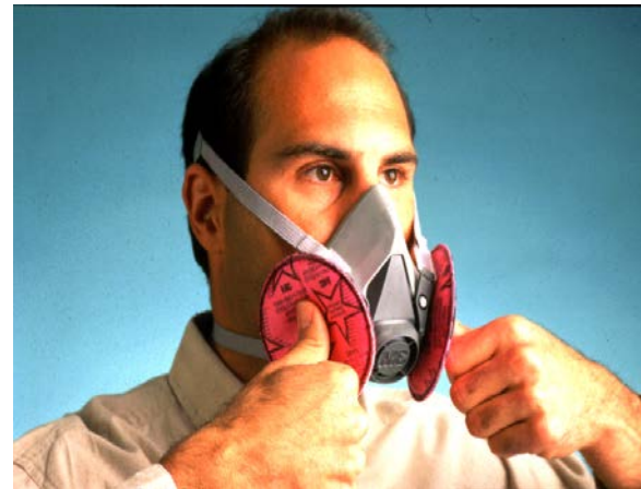
Negative Pressure Check
