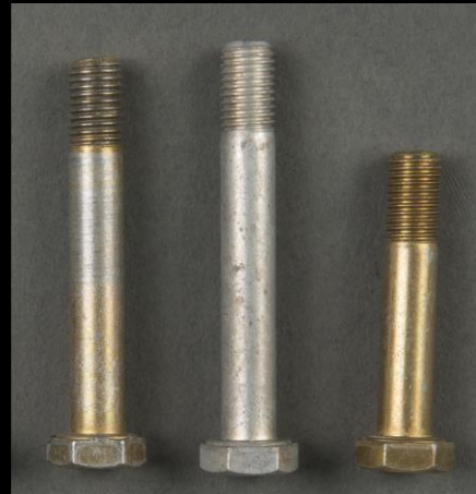
Cadmium-plated steel Military grade AN5 bolts
